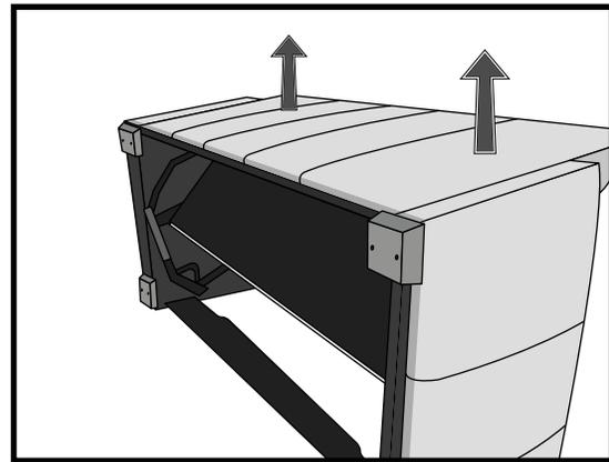
5. With the four bolts removed (from the previous step), the back can now be lifted away from the sleeper and set aside.
