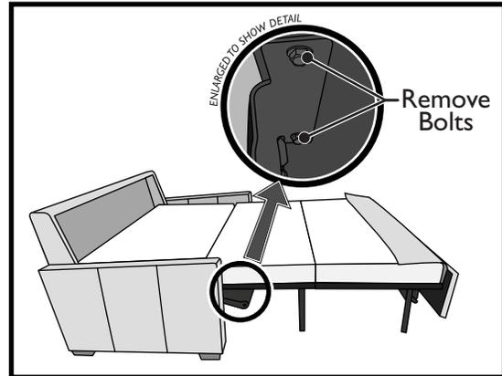
1. To begin, open the comfort sleeper as shown. Remove the two bolts connecting the middle bed section to the mechanism, as shown in the enlarged view. Do this on both the left and right sides.
