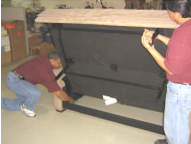
1. Open bed to this position and remove spring from each arm
