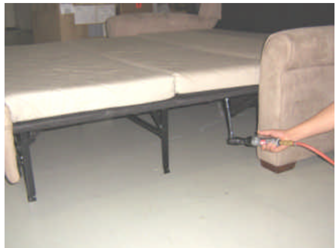
6. Open bed and remove the bolts shown in step 5
