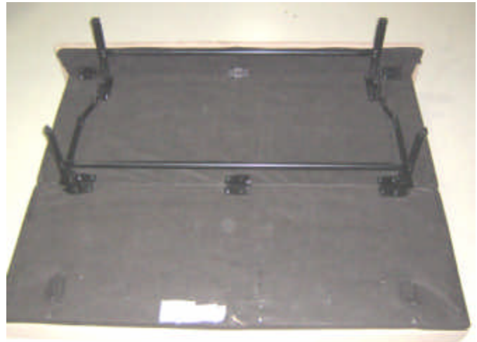
16. If leg mechanism needs to be replaced then place the front and middle bed sections face down on the floor, remove and reuse cross tubes when installing new mechanism
