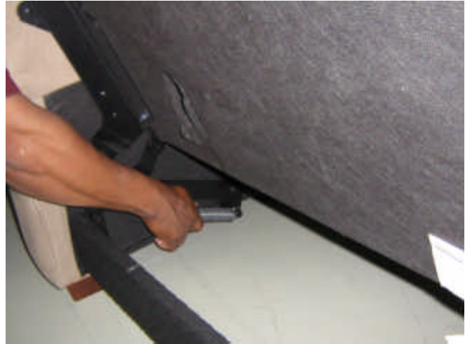
2. Position bed until the least amount of tension is on the spring. Grasp spring firmly and remove
