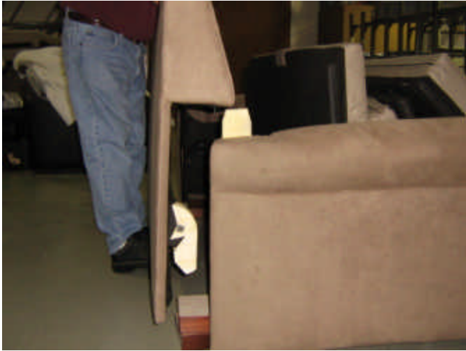
13. Lift Outside Back up and back to remove
