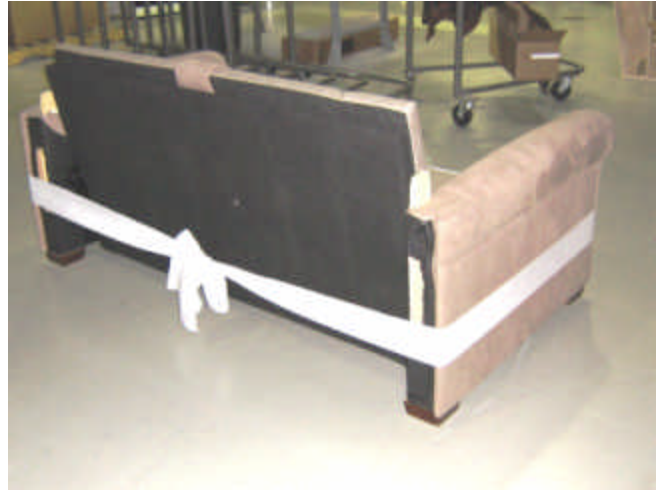
6. Tie the backs of the arms together. A shipping strap could be used if the leather / fabric are protected by a blanket / bag, or, replace the sofa bag, and tape around the sofa
