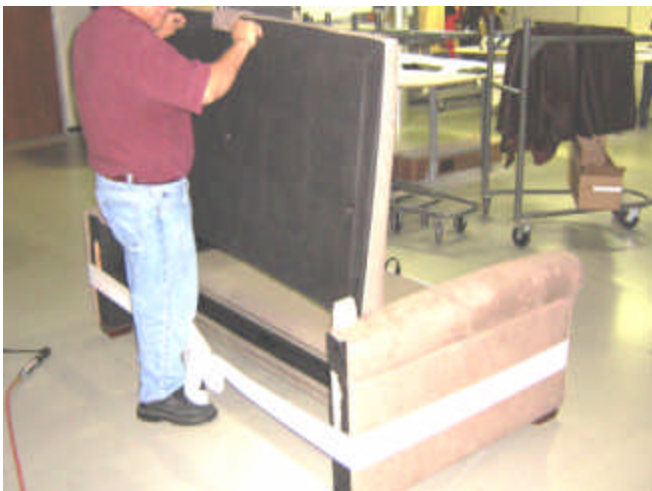
9. Lift back bed section out of frame
